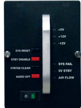
Vector System Monitor Integrated into removable power supply assembly
